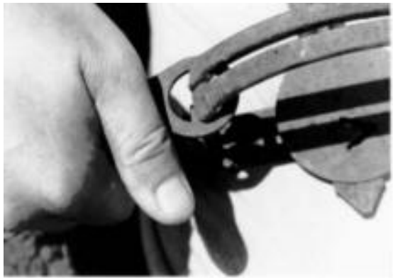
Fig. 13. Place one of the traps on your left leg just above your knee. Grasp the trap spring nearest your right leg as shown, and compress the spring.
