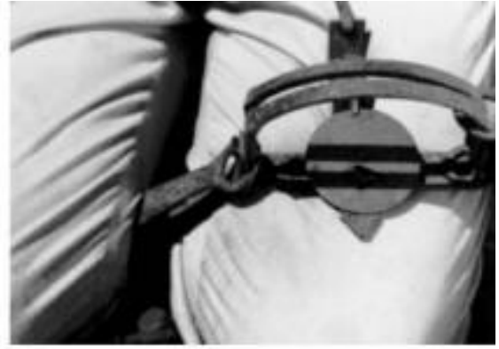
Fig. 15. Hold the compressed spring with your right leg as shown above, then compress the left spring. Hold this spring down with your left hand.
