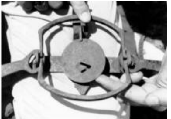
Fig. 16. Carefully spread the jaws. Reach under the jaws with your left hand, holding the pan up while you ease the two springs' tension so that the trap will remain set.
