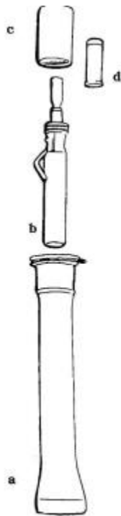
Fig. 8. The M-44 device consists of the (a) base, (b) ejector, (c) capsule holder, and (d) cyanide-containing plastic capsule.
