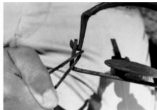
Fig. 14. Compress this spring below the jaw hinge, then bend the spring as shown above.
